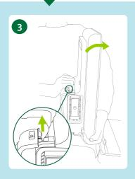
Hold the scanner unit securely while you reach inside the slot to release the safety bracket. The bracket may be warm.
